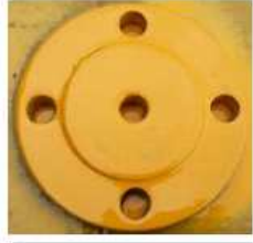
2. Painting Apply paint after 4 hours.
