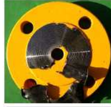
3. Remove CK-656 CK-656 is removed after complete hardening of paint.
