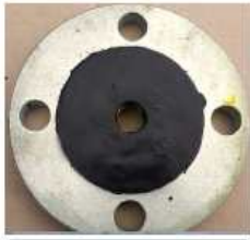
1. Apply CK-656 Apply using a brush (black)
