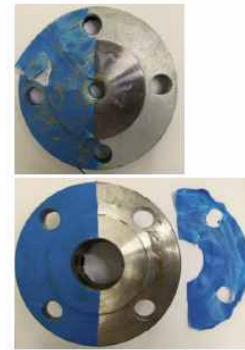
3. Remove CK-656 After drying for more than 4 hours, left for 168 hours Good surface condition
