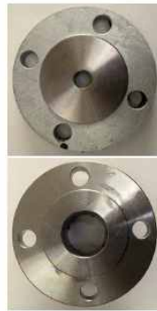
1. Flange preparation Remove impurities with Cleaner before testing.
